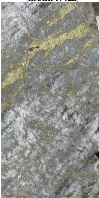
Diamond drill core from high grade quartz chalcopyrite stockwork veining (KPDH13 57-62m)
