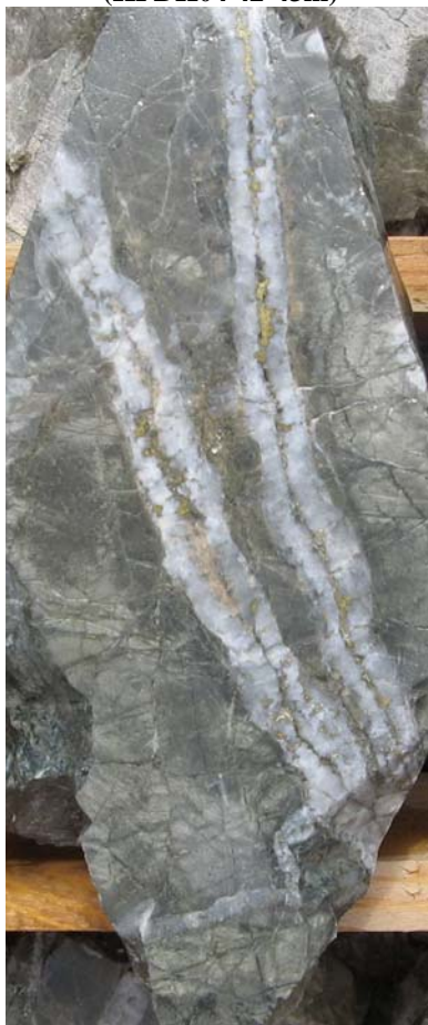
Diamond drill core from high grade quartz chalcopyrite stockwork veining (KPDH13 57-62m)
